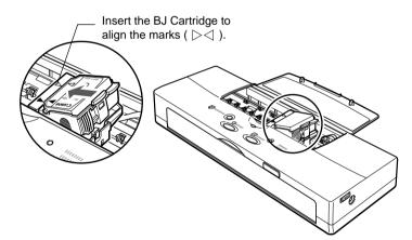
**10.** Press down on the high side of the BJ Cartridge until it snaps into the cartridge holder.
